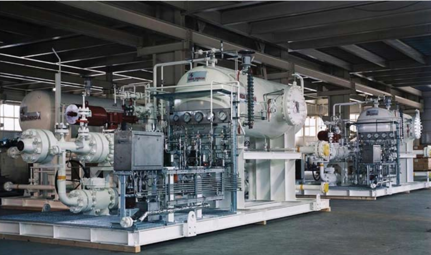
Wellhead Control and Methanol Injection Skid South and North Gas Exploration Project (Syria) STG Engineering Russia
